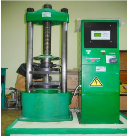
Figure 1. General view of hydraulic press \Pi -50 for determining deformation characteristics of the backfill material made of broken rock
